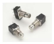
The single pole 110 and 641 series represent the most compact offerings of our pushbutton switch line. Rugged metal construction, self cleaning contacts and stiff actuation force (3-3 1/2 lbs. typical) have made these switches ideal for most "foot pedal" type applications. These alternate action switches fit a standard .500" mounting hole, have termination options including solder lug, wire lead and PC, and are popular within The Music Industry and Audio-visual market segments.
